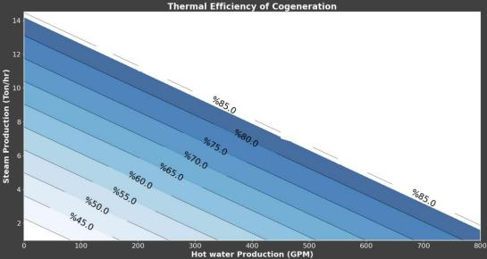
The plot above demonstrates the thermal efficiency of MPG power generation units when integrated with MSG steam and hot water generation units, as influenced by the volume of steam and hot water produced.
