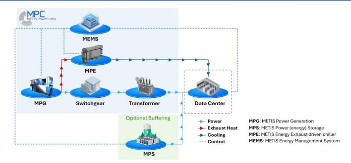
Our solution breaks the cycle of inefficiency by converting wasted exhaust heat into your most critical asset: cooling power. This integrated system pairs a extra low-emission gas turbine with an advanced exhaust-driven chiller, creating a unified power and cooling core for your data center.
